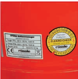
Electrical testing according to DIN
